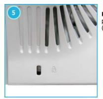
**Kensington Lock**: The Kensington lock is a device used to physically fix the system when using it in a public place. (The locking device has to be purchased separately.)
